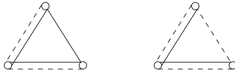
Figure 3: The two mixed circuits on three vertices. These graphs, denoted by K_3^+ and K_3^- , are the smallest (mixed) circuits of the direction-length rigidity matroid.
